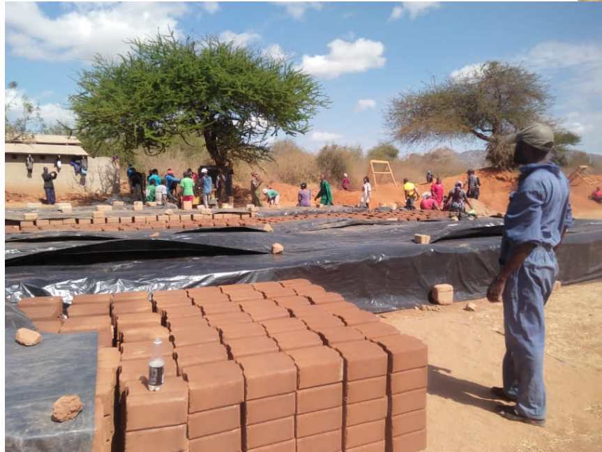
Production of ISSBs for construction of a school in Mikuyuni, Makueni
