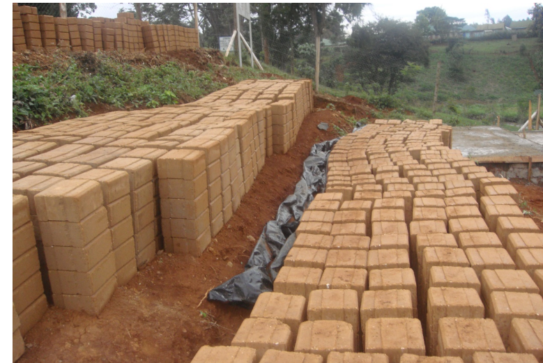
Interlocking Stabilized Soil Blocks
